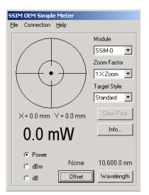
The Module selection box will allow you to select any SSIM that is currently connected.
