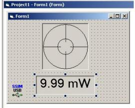
**4.1** Set the SSIMPower object to the desired size. Set the alignment property to the desired alignment. Adjust the font property to the desired font, size and style. Select the desired Display Mode (Power, dB or dBm). These properties can also be set at run time.
