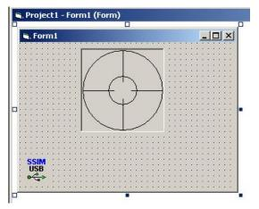
**3.1** Select the desired **Target Style**, **Border Style**, **Target Color** and **Dot Color** from the properties window. These properties can also be set at run time.
