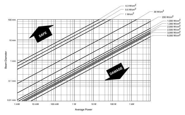
Variation of beam diameter and power for average power densities of thermal and semiconductor sensors. Safe operating limit above damage threshold lines.
